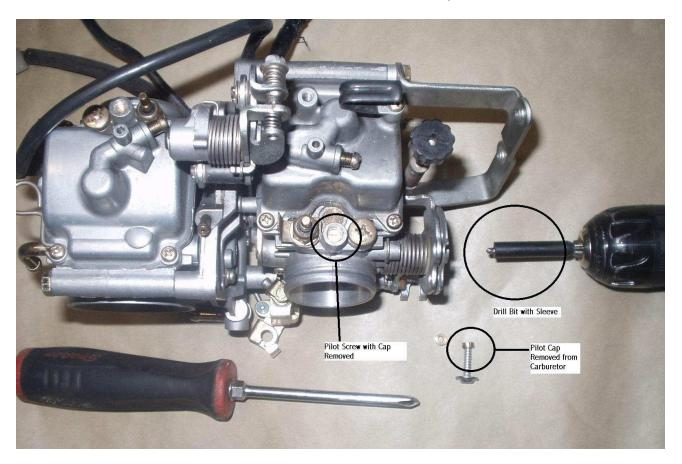
This picture shows the completed pilot cap removal including cleanup of metal filings before the carburetor bowls are removed. Tools are shown except the pliers used to pull the cap out after a screw was inserted in the drilled cap hole.
