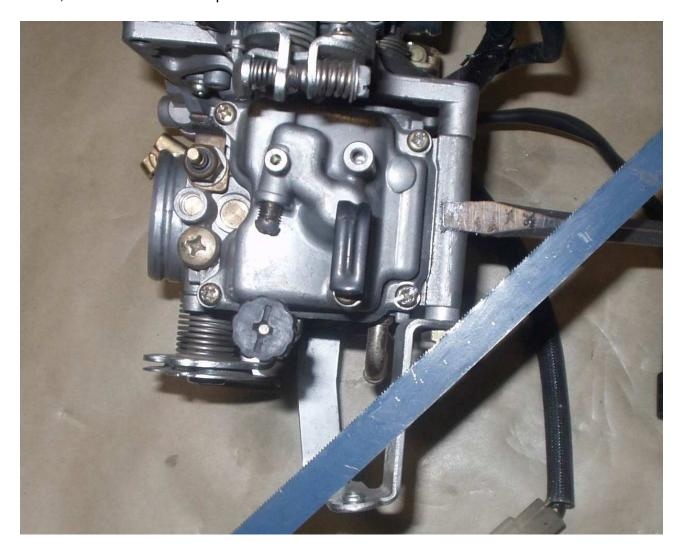
This carburetor has two stripped screws on the right side.
