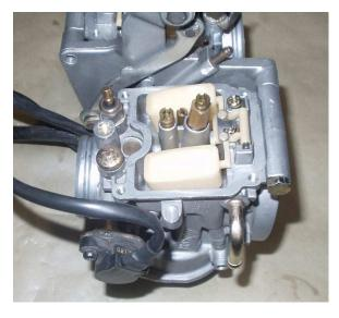
Here is a picture of the carburetor after the pilot cap has been removed, and the damaged bowl screws removed to open the carburetor for cleaning.
