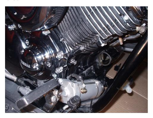
Clean and check the starter after it is removed. Look at the lineup marks and check for twist. Loosen the 8mm case bolts and twist the starter ends on the case to realign.
