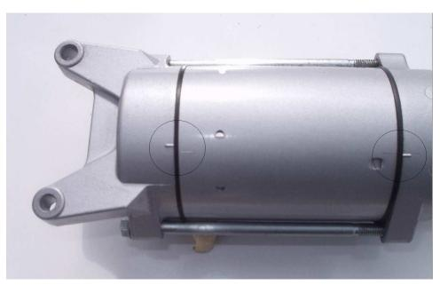
This picture shows a starter with a twisted case. It is not severe, but the bolts are slightly bent.
